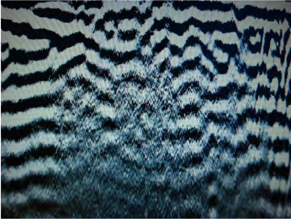
GPR images over target D showing stratigraphic walls delineating altered and unaltered soils
