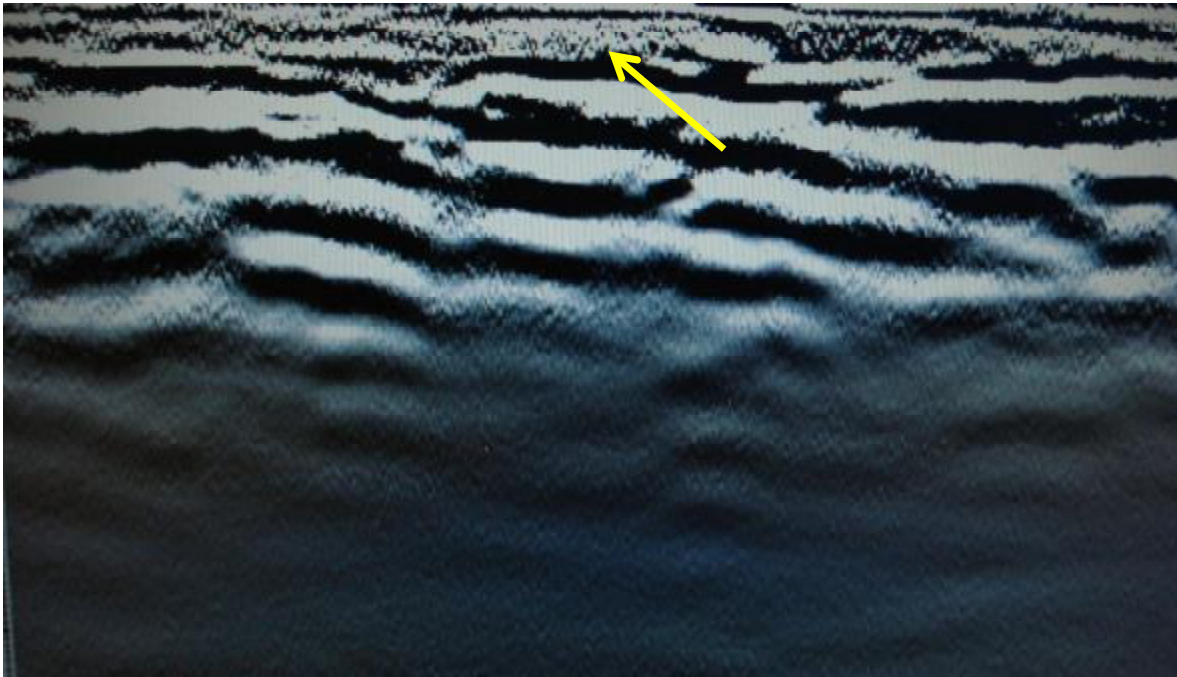
Saturated ground from recent rains making data less clear small anomalies from rebar in concrete pad Target A
