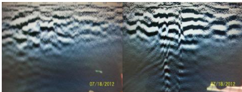
GPR images from transect passes over and near targets N and P
