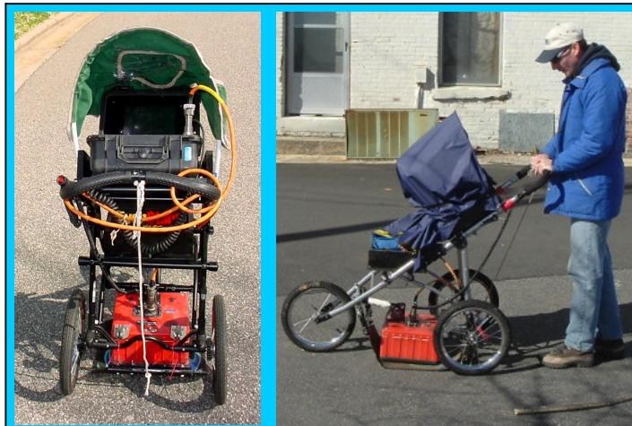
The photographs show the SIR-2000 GPR system equipped with a 400 MHz antenna that were used to conduct the ground penetrating radar investigation across selected EM61 differential anomalies at the Parcel 12 site on August 21, 2012.
