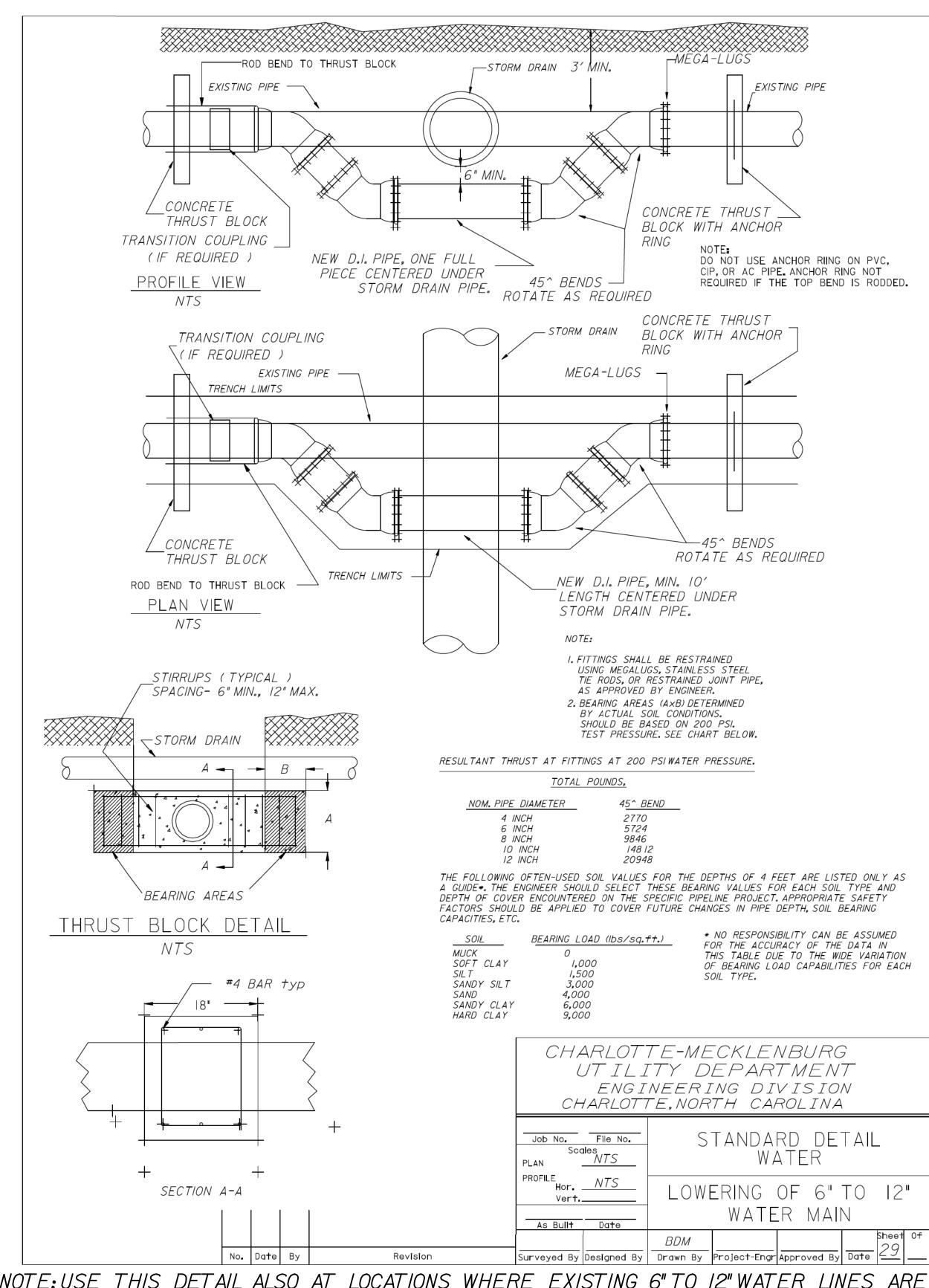
NOTE: USE THIS DETAIL ALSO AT LOCATIONS WHERE EXISTING 6"TO 12" WATER LINES ARE RELOCATED.
