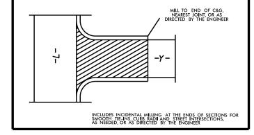
MILLING AT CURB AND GUTTER INTERSECTIONS
