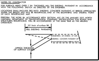
MILLING AT PAVEMENT TIE-INS DETAIL
