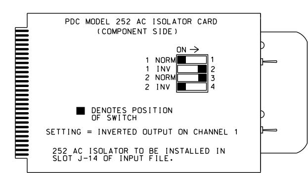
NOTE: IF ANOTHER MANUFACTURER TYPE OF AC ISOLATOR IS USED, OUTPUT PROGRAMMING IS LIKELY NOT TO EQUATE TO THAT SHOWN ABOVE.
