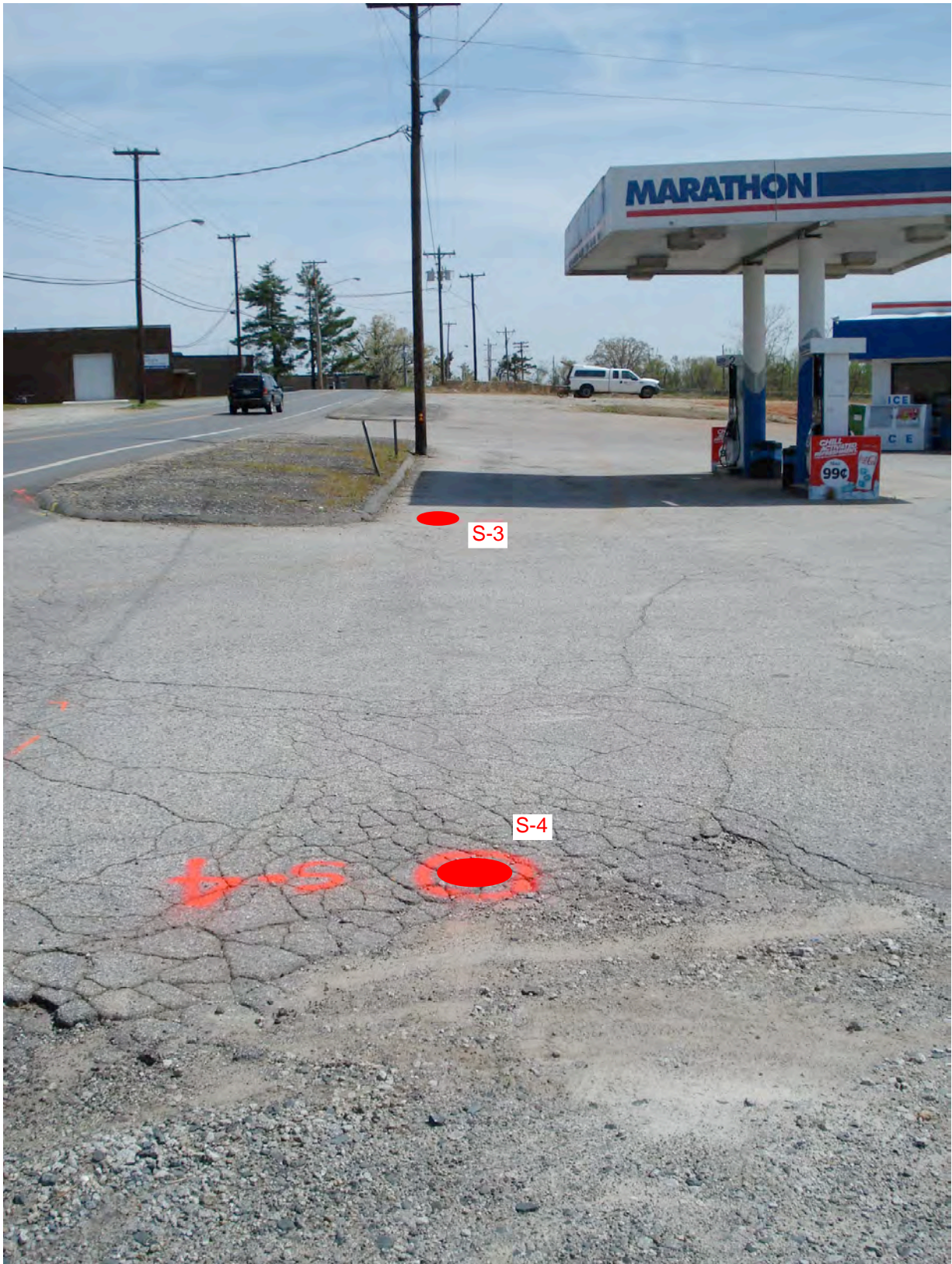
Photograph 5 : View looking east at locations of soil borings S-3 and S-4. Metal posts that produced linear EM-61 image shown in Figure 3 are shown in background.
