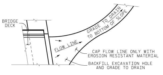
IF THE APPROACH SLAB IS NOT CONSTRUCTED IMMEDIATELY AFTER THE BACKFILLING OF THE END BENT EXCAVATION, GRADE TO DRAIN TO THE BOTTOM OF THE SLOPE AND PROVIDE EROSION RESISTANT MATERIAL, SUCH AS FIBERGLASS ROVING OR AS DIRECTED BY THE ENGINEER TO PREVENT SOIL EROSION AND TO PROTECT THE AREA ADJACENT TO THE STRUCTURE. THE CONTRACTOR WILL BE REQUIRED TO REMOVE THESE MATERIALS PRIOR TO CONSTRUCTION OF THE APPROACH SLAB.
