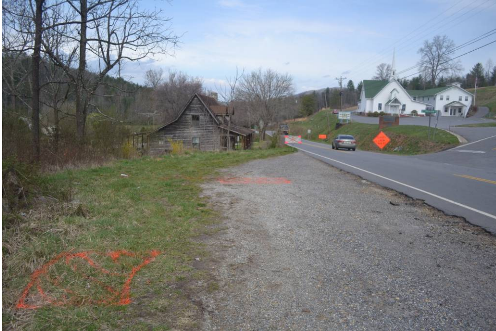
Photograph 1: Two geophysical anomalies identified at NCDOT Parcel 19 by GPR and demarcated in orange paint on April 4, 2014. Area demarcated in orange paint on left above did not appear to contain a UST (push-probe extended to four feet bgs). View is to the northwest parallel to NC 294. Friendship Church Road can be seen to the right.
