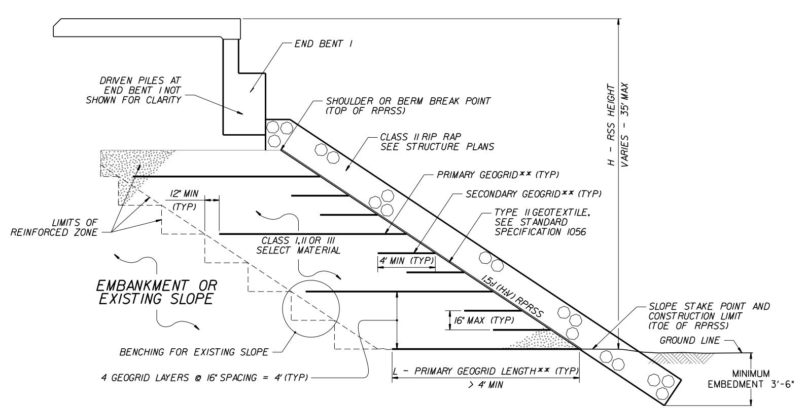
EB1 END SLOPE RPRSS WITH SELECT MATERIAL THAT DOES NOT MEET ARTICLE 1019–2 OF THE STANDARD SPECIFICATIONS
