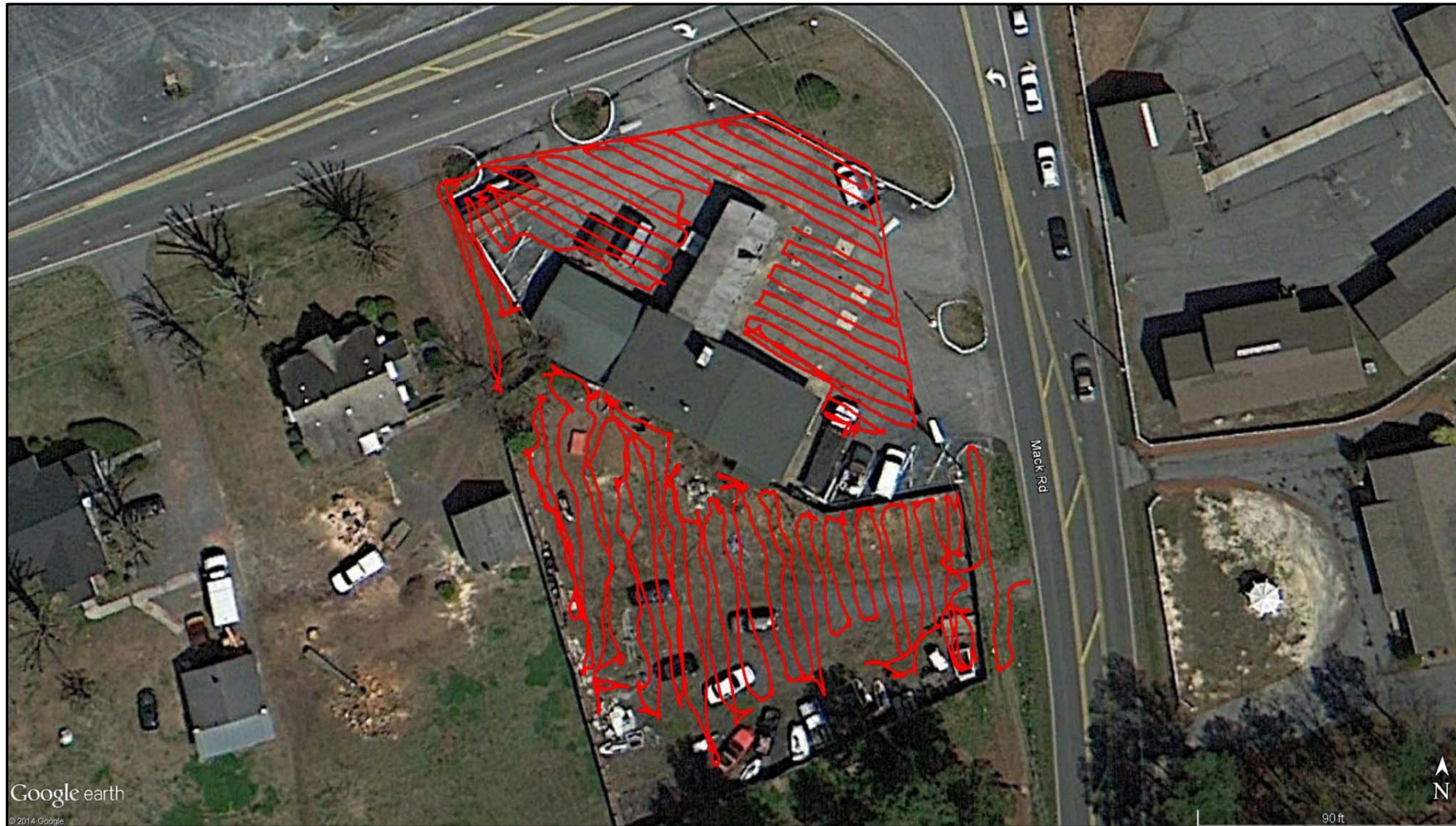
Red Line Indicates Path of EM61 Across Survey Area
