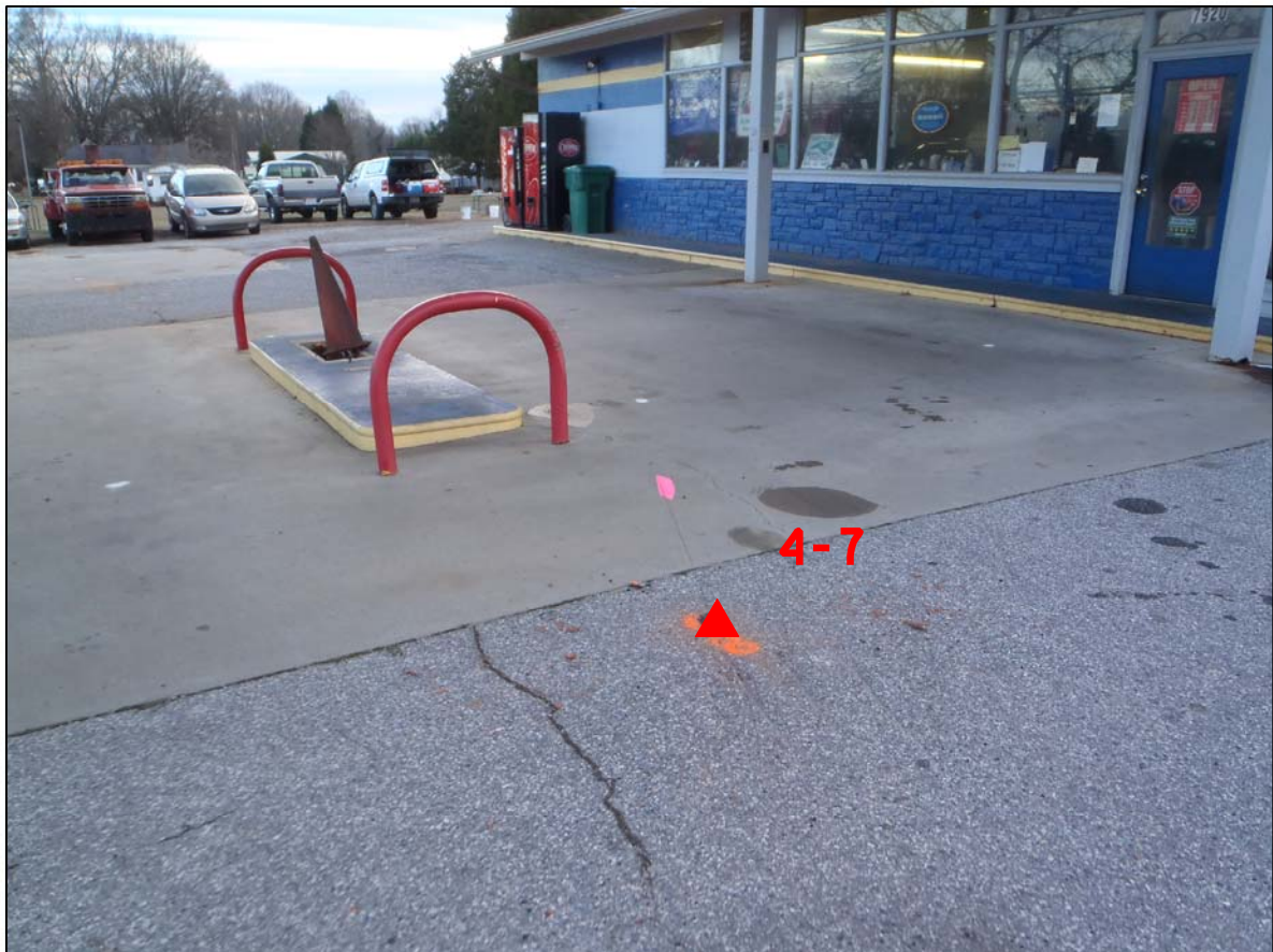
PHOTO 8 - BORING AT FORMER PUMP ISLAND LOOKING SOUTH
