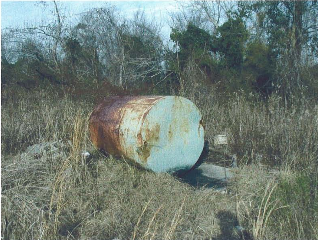
Photograph No. 7: Abandoned AST north of the garage. The concrete was stained with oil below the tank.
