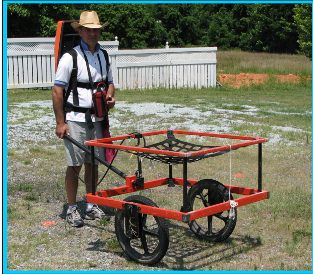
The photograph shows the Geonics EM61 metal detector that was used to conduct the metal detection survey across the southern portion of the Jerry McKinney property on February 7, 2012. Due to an absence of unexplained EM61 differential anomalies, ground penetrating radar scans were not performed at this site.
