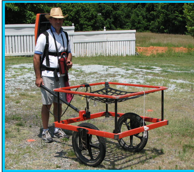
The photograph shows the Geonics EM61 metal detector that was used to conduct the metal detection survey across the southern portion of the Calvary Assembly of God of Spruce Pine property on February 7, 2012. Due to an absence of unexplained EM61 differential anomalies, ground penetrating radar scans were not performed at this site.
