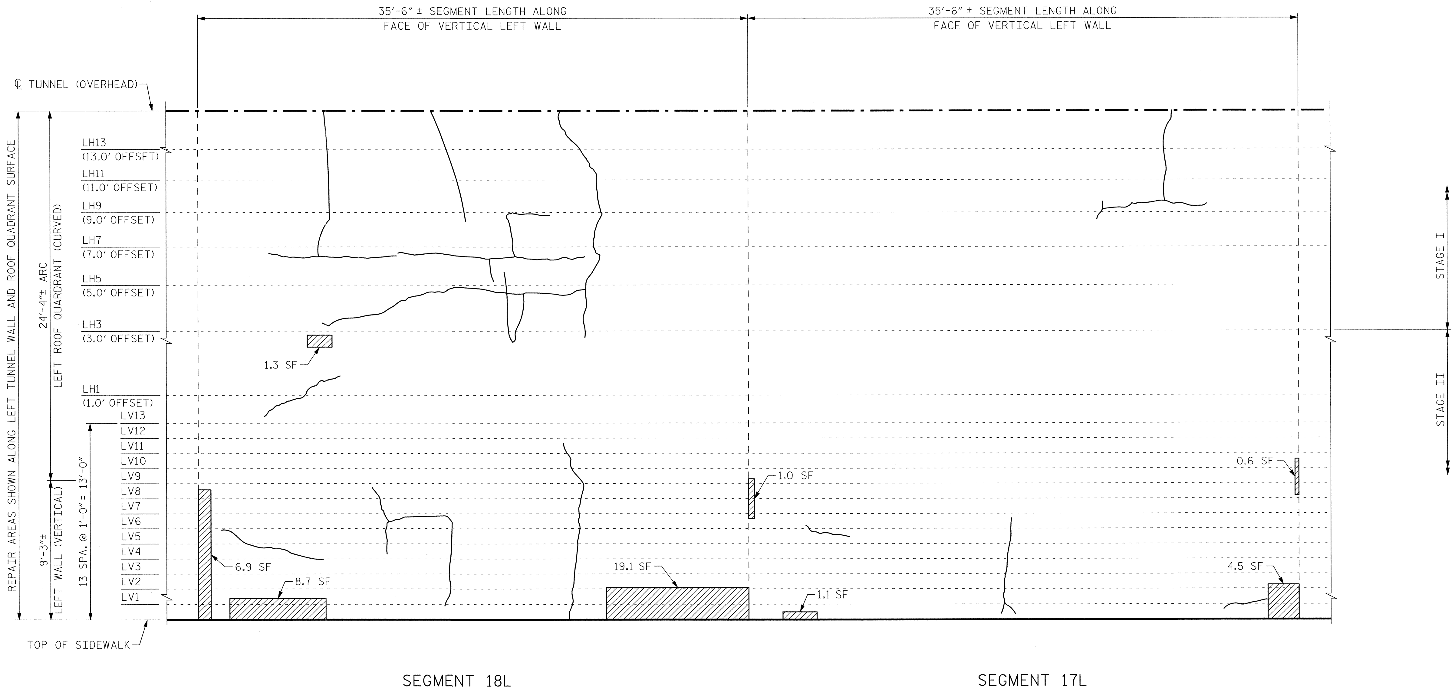
VIEW B-B: REPAIR SEGMENTS 17L & 18L TUNNEL SURFACE ELEVATION
