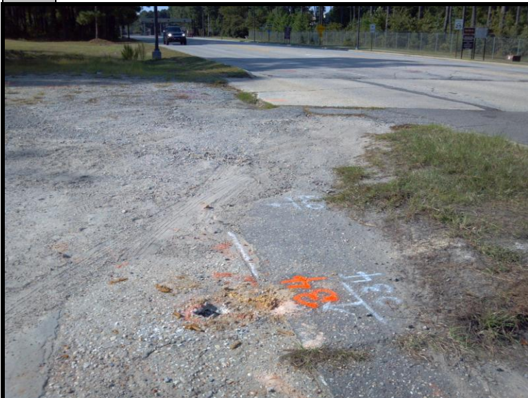
7 Boring B-4. The boring was advanced to 45 ft. bgs, but no water was encountered. See text for details.
