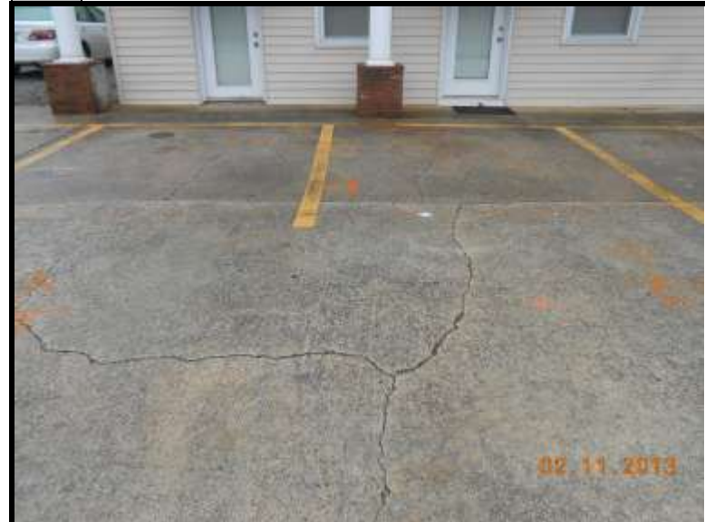
View of Anomaly 1 with probable UST's outlined with orange spray paint. View is to the northwest.
