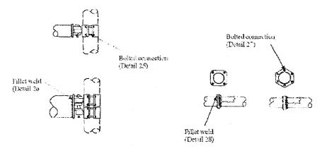
Beam-Column Cornection for monotube structure Example 16
