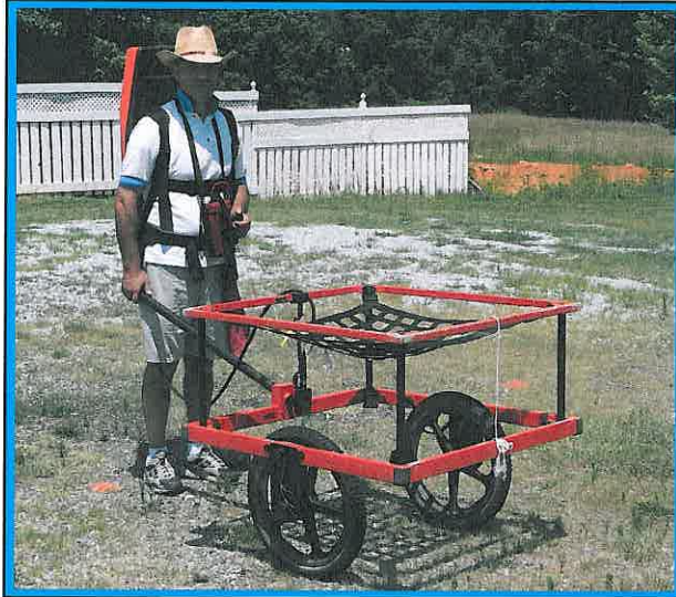
The photograph shows the Geonics EM61 metal detector that was used to conduct the metal detection survey across the proposed Right-of-Way area at Parcel 182 on November 10, 2011. Due to an absence of unexplained EM61 differential anomalies, ground penetrating radar scans were not performed at this site.
