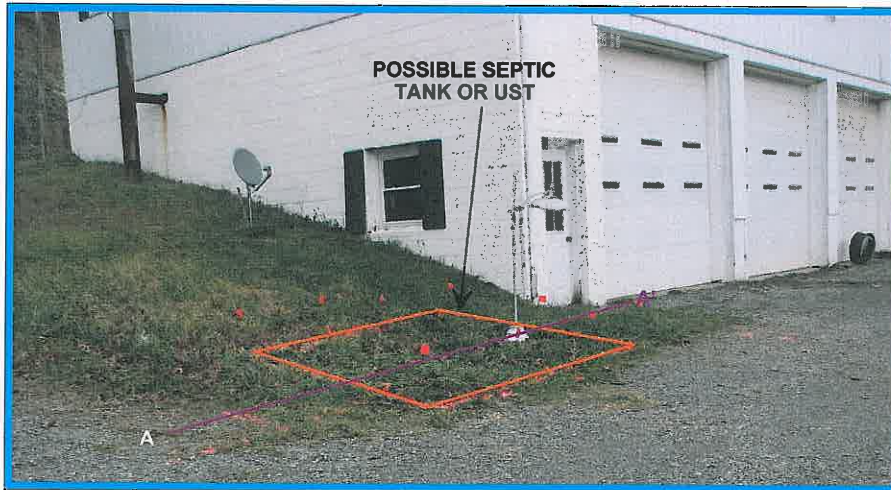
The orange rectangle in the photograph represents the approximate perimeter of a possible septic tank or UST or other miscellaneous object, as suggested by the GPR data. Centered near grid coordinates X=46 Y=350, the tank or object is approximately 9 feet long, 6.5 feet wide and buried 2 feet below present grade. The solid purple line in the photograph represents the approximate location of the GPR image shown above. The photograph is viewed in a southeasterly direction.
