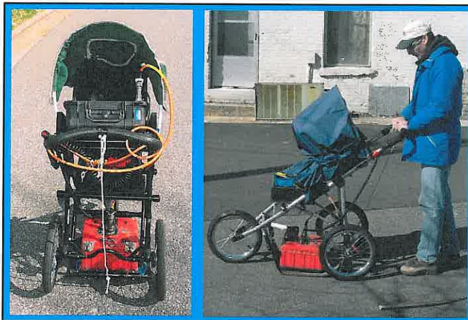
The photographs show the SIR-2000 GPR system equipped with a 400 MHz antenna that were used to conduct the ground penetrating radar investigation across selected EM61 differential anomalies at Parcel 141 on November 17, 2011.
