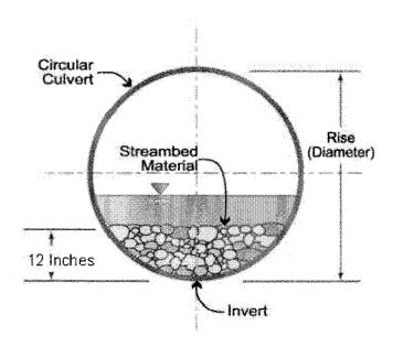
In all other counties: Culverts greater than 48 inches in diameter will be buried at least one foot below the bed of the stream. Culverts 48 inches in diameter or less shall be buried or placed on the stream bed as practicable and appropriate to maintain aquatic passage, and every effort shall be made to maintain the existing channel slope. The bottom of the culvert must be placed at a
