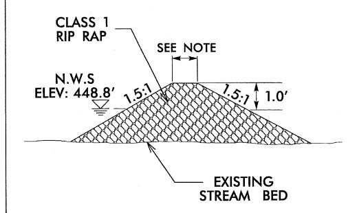
NOTE: CAUSEWAY WIDTH SHALL BE EXISTING BRIDGE WIDTH PLUS 5' ON EACH SIDE.
