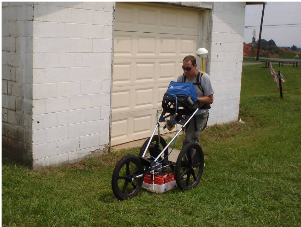
GSSI SIR-3000 Ground-Penetrating Radar with 400 MHz Antenna
