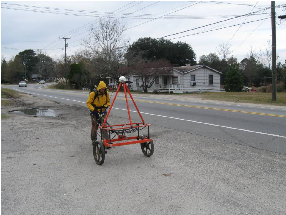
Geonics EM61-MK2 Metal Detector with Trimble DGPS Unit
