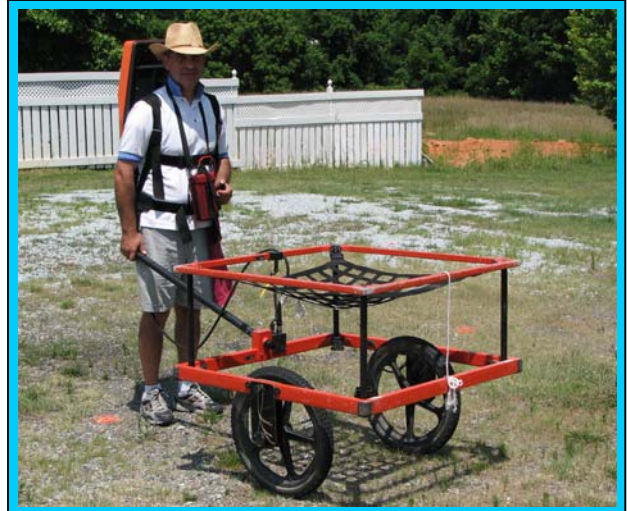
The photo shows the Geonics EM61 metal detector that was used to conduct the metal detection survey at Parcel 4 on June 26, 2007.
