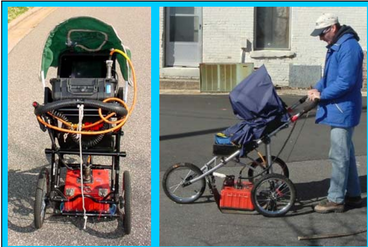
The photos show the SIR-2000 GPR system equipped with a 400 MHz antenna that were used to conduct the ground penetrating radar investigation at Parcel 4 on June 27, 2007.
