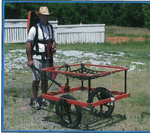
The photograph shows the Geonics EM61 metal detector that was used to conduct the metal detection survey across the geophysical survey area at the Hico Joan, LLC property (Parcel 154) on June 25, 2010.
