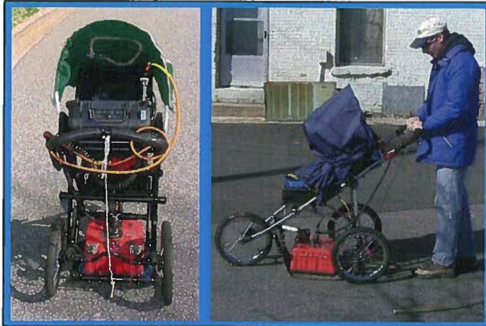
The photographs show the SIR-2000 GPR system equipped with a 400 MHz antenna that were used to conduct the ground penetrating radar investigation at Parcel 122 on June 30, 2010.
