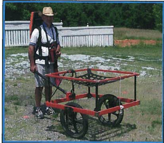
The photograph shows the Geonics EM61 metal detector that was used to conduct the metal detection survey across Parcel 122 on June 28, 2010.
