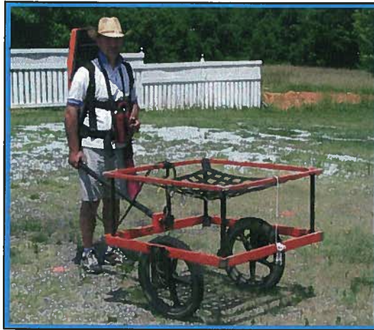
The photograph shows the Geonics EM61 metal detector that was used to conduct the metal detection survey across the FFCA/IPI property (Parcel 108) on June 24, 2010.
