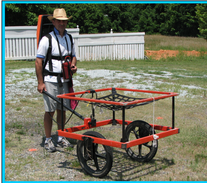
The photograph shows the Geonics EM61 metal detector that was used to conduct the metal detection survey across the proposed ROW area at the Matthews Oil Company Inc. property on July 22, 2010.
