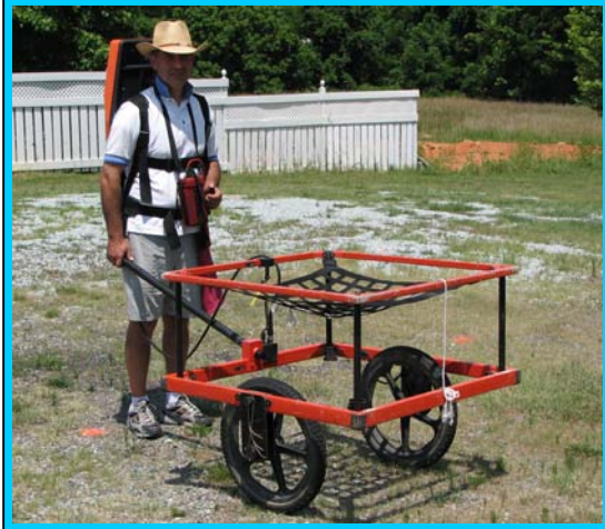
The photograph shows the Geonics EM61 metal detector that was used to conduct the metal detection survey across the proposed ROW areas at the Ruby Tuesday Inc. property on July 22, 2010.
