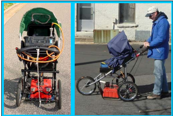
The photographs show the SIR-2000 GPR system equipped with a 400 MHz antenna that were used to conduct the ground penetrating radar investigation at the Claude Meachum property on August 3, 2010.
