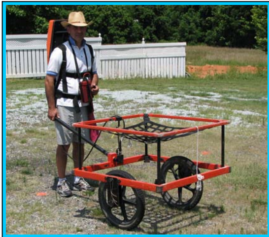
The photograph shows the Geonics EM61 metal detector that was used to conduct the metal detection survey across the proposed ROW area at the Claude Meachum property on July 22, 2010.
