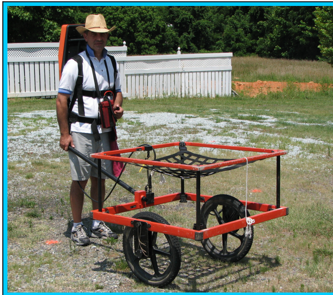
The photograph shows the Geonics EM61 metal detector that was used to conduct the metal detection survey across the proposed ROW area at the Willie Brantely site on July 21, 2010.
