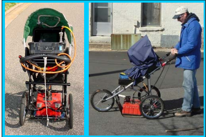
The photographs show the SIR-2000 GPR system equipped with a 400 MHz antenna that were used to conduct the ground penetrating radar investigation at the Mary Spires property on August 2, 2010.
