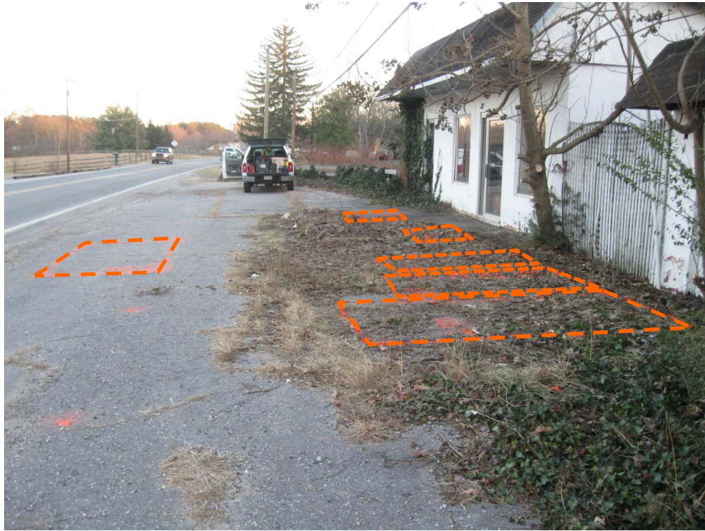
Parcel 87 – Olaf & Valeria Adams Property, looking southeast. Photo shows approximate marked location of the probable USTs on the east side of the property.
