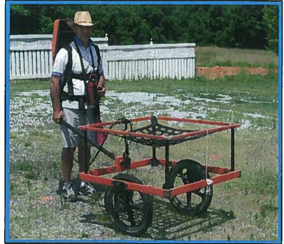
The photograph shows the Geonics EM61 metal detector that was used to conduct the metal detection survey at Parcel 168 on October 22, 2010.
