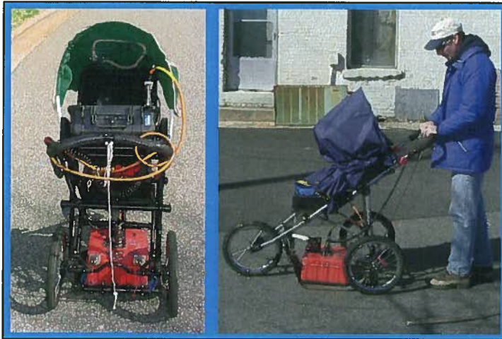
The photographs show the SIR-2000 GPR system equipped with a 400 MHz antenna that were used to conduct the ground penetrating radar investigation at Parcel 168 on October 29, 2010.
