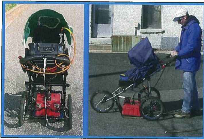
The photographs show the SIR-2000 GPR system equipped with a 400 MHz antenna that were used to conduct the ground penetrating radar investigation at Parcel 147 on October 29, 2010.
