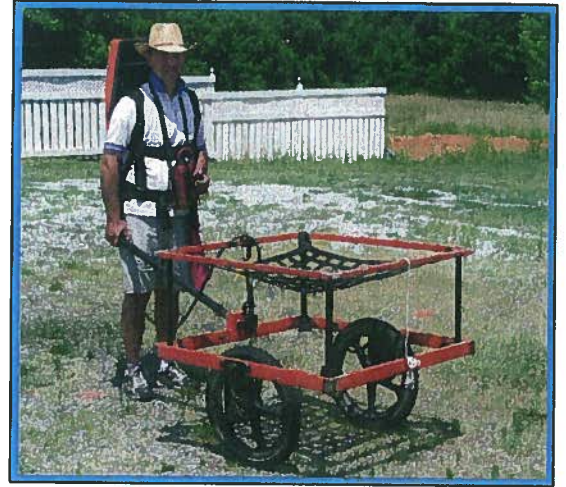
The photograph shows the Geonics EM61 metal detector that was used to conduct the metal detection survey at Parcel 147 on October 21, 2010.
