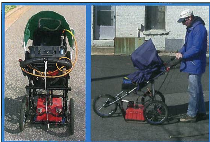
The photographs show the SIR-2000 GPR system equipped with a 400 MHz antenna that were used to conduct the ground penetrating radar investigation at Parcel 142 on October 29, 2010.
