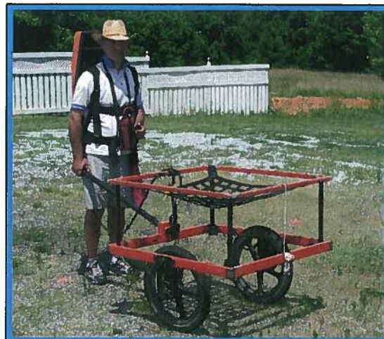
The photograph shows the Geonics EM61 metal detector that was used to conduct the metal detection survey at Parcel 142 on October 21, 2010.
