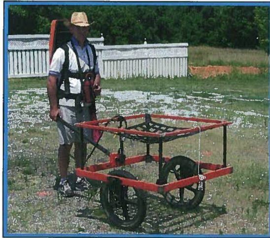
The photograph shows the Geonics EM61 metal detector that was used to conduct the metal detection survey across Parcel 19 on October 22, 2010.
