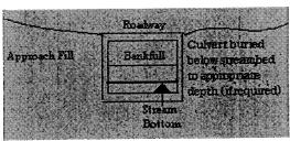
In all other counties: Culverts greater than 48 inches in diameter will be buried at least one foot below the bed of the stream. Culverts 48 inches in diameter or less shall be buried or placed on the stream bed as practicable and appropriate to maintain aquatic passage, and every effort shall be made to maintain the existing channel slope. The bottom of the culvert must be placed at a depth below the natural stream bottom to provide for passage during drought or low flow conditions.
