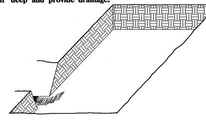
3. Backfill the trench with 50mm well rotted sawdust. Place a 50mm layer of well rotted sawdust at a sloping angle at one end of the trench.
