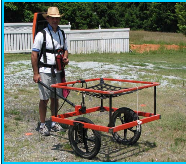
The photograph shows the Geonics EM61 metal detector that was used to conduct the metal detection survey across the accessible portions of the proposed Right-of-Way area at Parcel 51 on February 4, 2010.
