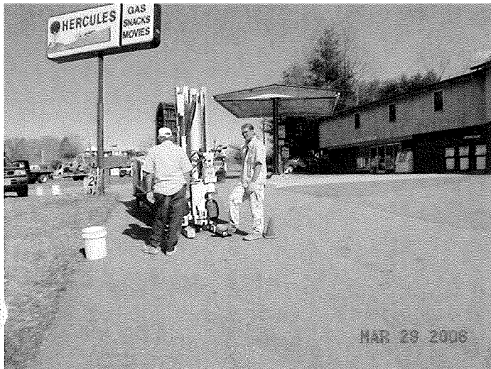
Photograph 5: Soil boring activities at GP-10 location downgradient of current UST systems.
