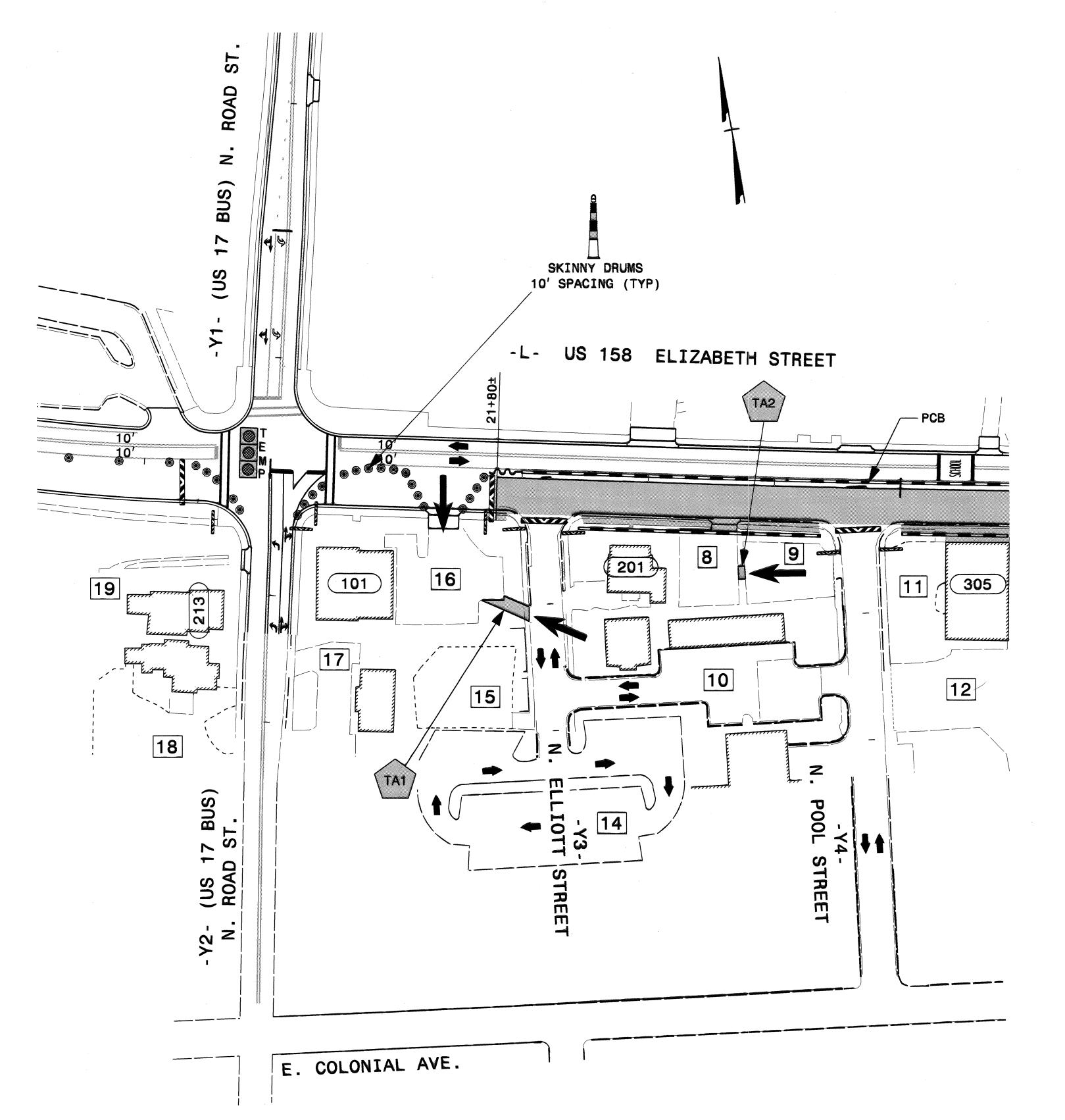
DURING PHASE III OF CONSTRUCTION SOUTHERN ACCESS TO ELIZABETH STREET WILL ONLY BE PERMITTED AT N. ROAD STREET AND PARKING AREA 16 WITHIN THE VICINITY OF THE DETAIL SHOWN ON PED-3. N. POOL STREET WILL BE CONVERTED TO A 2-LANE, 2-WAY TRAFFIC PATTERN. PARKING ALONG N. POOL STREET WILL NOT BE PERMITTED DURING THIS PHASE OF CONSTRUCTION.
