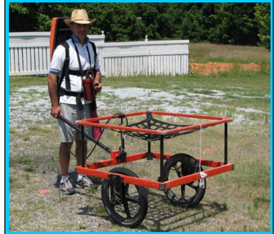
The photograph shows the Geonics EM61 metal detector that was used to conduct the metal detection survey across the 229 North Water Street site (Value Mart, Inc. property) on July 7, 2010.
