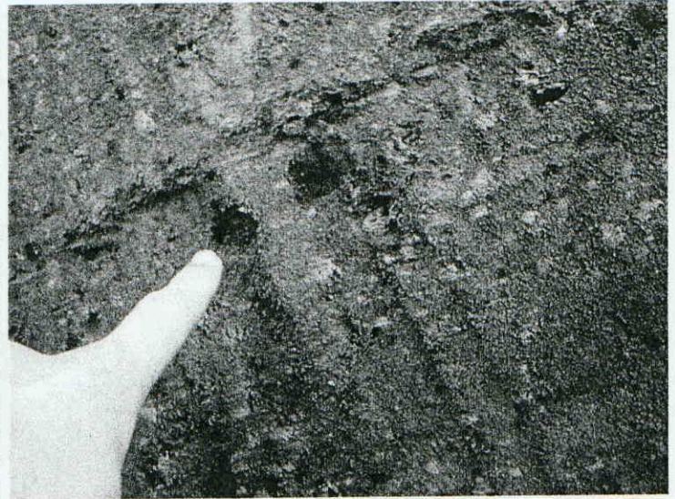
02060548 Former Esso/Exxon (Register Property) Tank #2-All USTs had small pits but no holes
