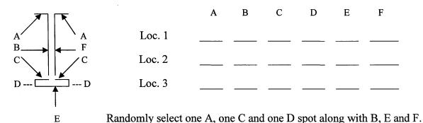
**B.** Two random adhesion tests per span are conducted on interior surfaces after the paint has been properly cured, and will be touched up by the Contractor. One random Cut Tape adhesion test per span is conducted on interior surface after the finish coat is cured, and
