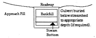
In all other counties: Culverts greater than 48 inches in diameter will be buried at least one foot below the bed of the stream. Culverts 48 inches in diameter or less shall be buried or placed on the stream bed as practicable and appropriate to maintain aquatic passage, and every effort shall be made to maintain the existing channel slope. The bottom of the culvert must be placed at a depth below the natural stream bottom to provide for passage during drought or low flow conditions.
