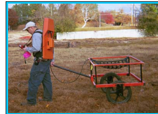
The photo shows the Geonics EM61 metal detector that was used to conduct the metal detection survey at the sites in Richmond County, North Carolina.
