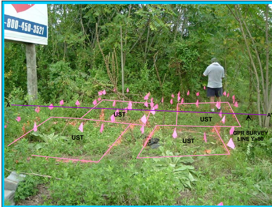
The photograph shows the location of four probable USTs buried 1.75 to 2.0 feet below surface, as suggested by the geophysical results at Parcel 21.
