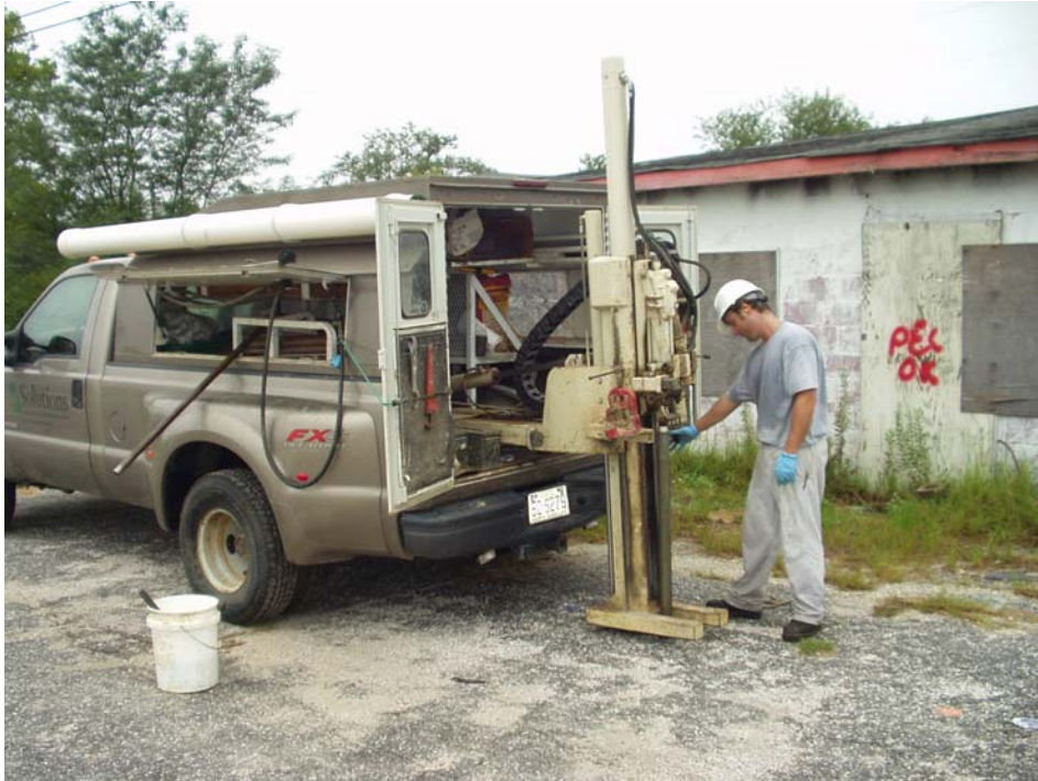
Photograph 2 – Advancing a soil boring with the Geoprobe®.
